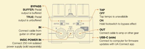
**Power Supply** Isolated 9VDC, center-negative, 250 mA minimum, 2.1x5.5 mm barrel connector (sold separately)
