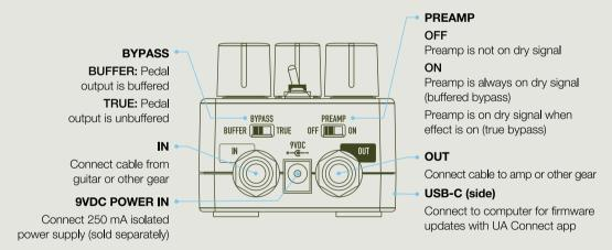
**Power Supply** Isolated 9VDC, center-negative, 250 mA minimum, 2.1x5.5 mm barrel connector (sold separately)
