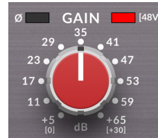
Channel 2 GAIN Relay enabled
