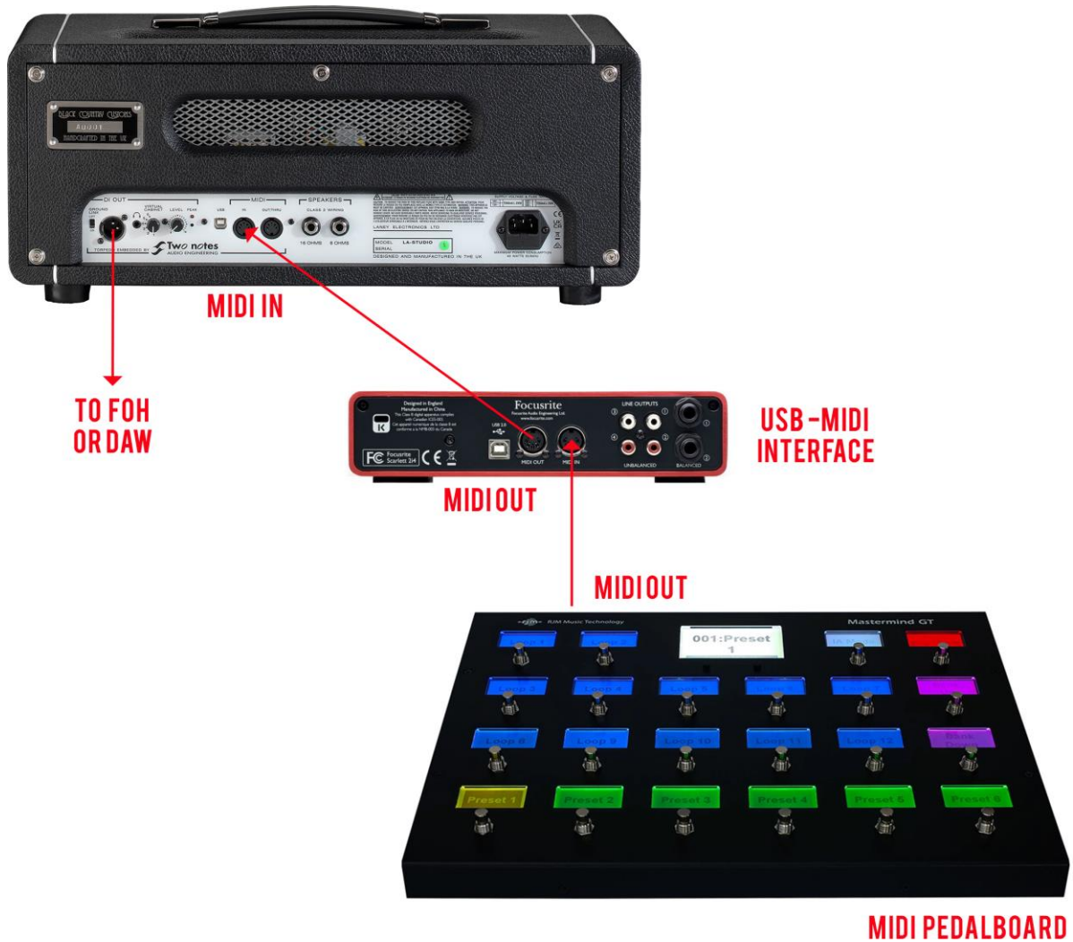
Figure 4 LA-STUDIO guitar into head, head into FOH, USB-MIDI interface & MIDI pedal board
