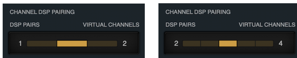
Channel DSP Pairing control as it appears with Apollo Twin (left) and Apollo rackmount models (right)
