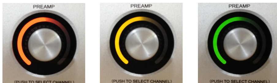
The color of Apollo's preamp gain level indicator changes to reflect the gain stage being controlled
